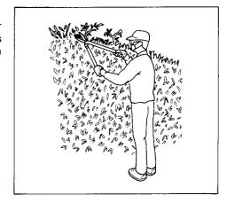
Hold the tool firmly with both hands. Switch on the tool without the blades making any contact. Move the tool in front of your body while cutting.
